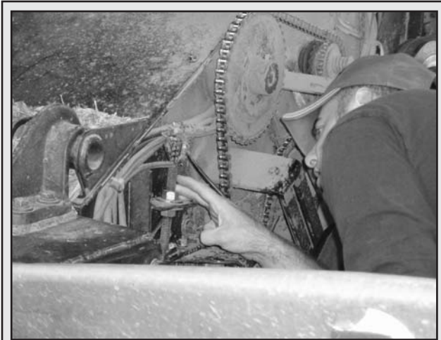
Figure 2. A member of the Student Agriculture Association Team adjusts the concave and cylinder distance on an Allis Chalmers Gleaner model F3 plot combine to minimize grain loss during harvest.
