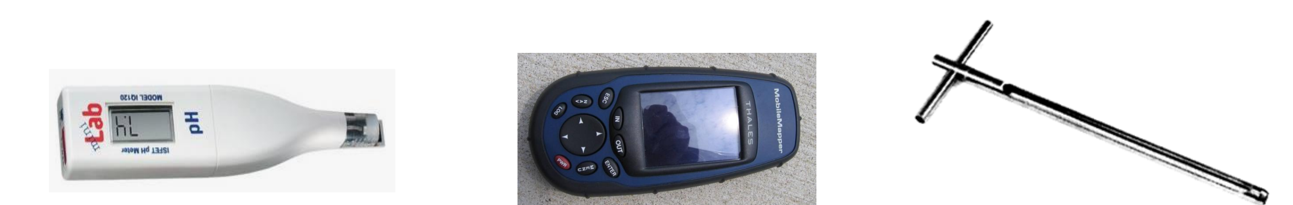
Figure 3 : pH meter, GPS Mobile Mapper and Soil Probe
