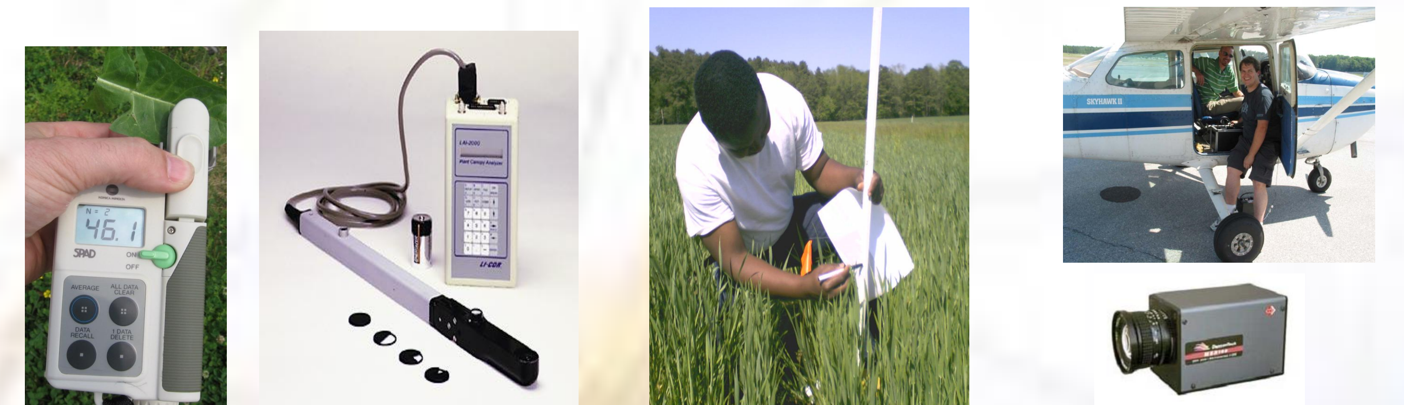
Figure 5 : SPAD meter, LAI meter, linear scale, CIR/RGB camera mounted on Cessna 172
