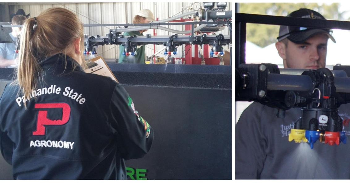
Spraying. A selection of spray nozzles was provided for identification using iPads loaded with the Nozzle Select app. Calculations covered sprayer calibrations and pulsewidth modulation. The ExactApply™ spray table was used for demonstrations in the situational analysis section.
